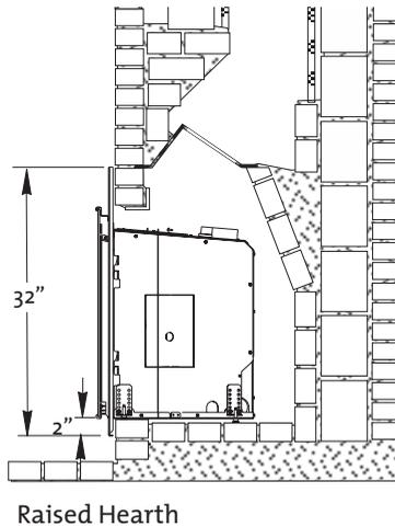
Adjustable riser brackets allow use of two different surround sizes to accommodate a variety of fireplace configurations.
